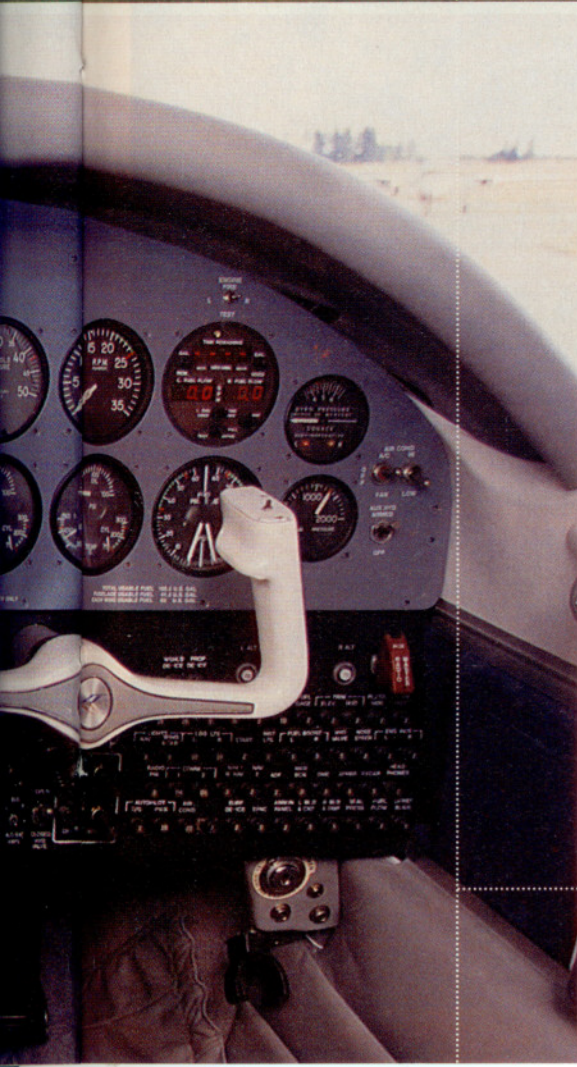
The Aerostar's instrument panel proves roomy enough for basic avionics, but the gadget-obsessed may feel slighted. Triple fuel gauges (above radio stack) came as part of an AD.
