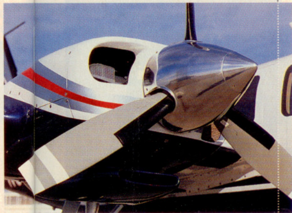
Piper-built 700Ps use 350-hp Lycomings and booted, three-blade props. Condition of the engines and accessories is a critical pre-buy focus.
