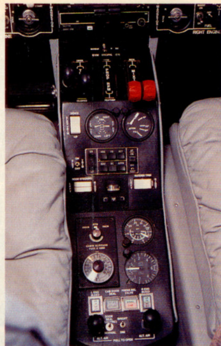
Pressurization controls inhabit the center console. Generally, the layout of the Aerostar cockpit is straightforward and easy to learn.
